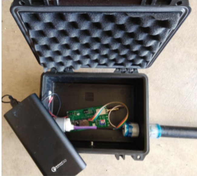
Figure 3: Sensor node configuration
