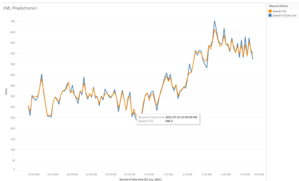
Figure 14: Timeseries plot of 15-second-ahead predicted wind speeds (orange) vs true wind speed (blue).
