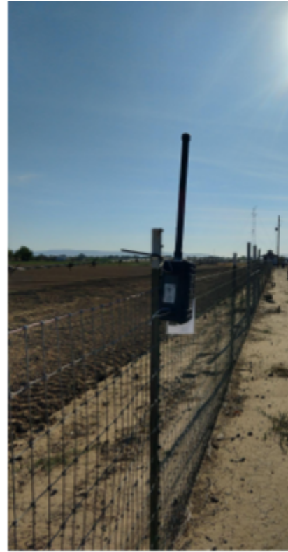
Figure 4: Typical sensor node installation at the Campbell Tract
